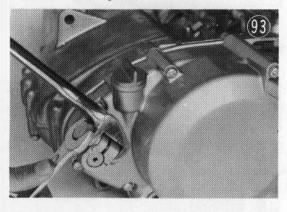
Remove the distributor cap mounting clamp, and the distributor cap. (H1 CDI only)
