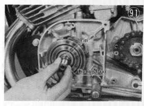
3. Align the projection on the engine sprocket lock washer with the hole in the sprocket, tighten down the mounting nut, and bend up one side of the lock washer.
