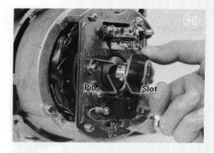
2. H1 (no CDI) - Align the timing cam slot with the pin on the rotor when mounting it.
