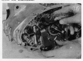
Take out the hex-head mounting bolt, and remove the set lever and spring
