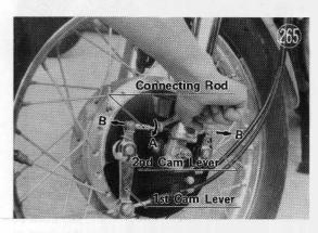
(ii) The second cam is now in the position shown in Fig. 266. Measurement "a" is the second cam's play, this amount being sufficient to avert second shoe contact with the drum when the front brake is operated.
