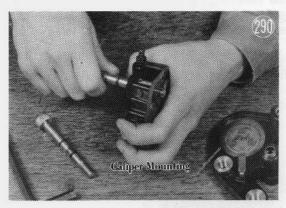
Loosen the two allen head shafts (10 mm allen wrench) as they will be difficult to loosen once the calipers are taken off the fork. Remove the two mounting bolts and take off the caliper assembly.
