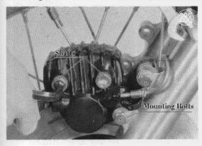
Take the band and dust seal off the piston. Blow compressed air into the caliper inlet to push out the piston. If compressed air is not available, reconnect the brake line and pump the piston out with the brake lever.
