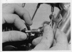
Pull the caliper mounting off the shafts evenly, being careful not to damage the shafts, O rings or seals. Take out the shafts.
