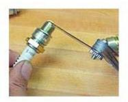
The standard plug is an NGK B-9HS-10. Plug installation torque is  $18.0 \sim 22.0$  ft-lb ( $2.5 \sim 3.0$  kg-M).
