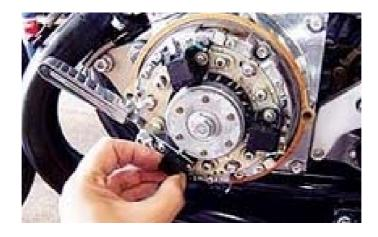
For precise timing adjustment, base plate must become parallel to an IG signal coil. Set the base plate as parallel to the base of the IG signal coil.
