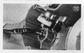
CAUTION: Do not remove the oil seal unless it is damaged.
