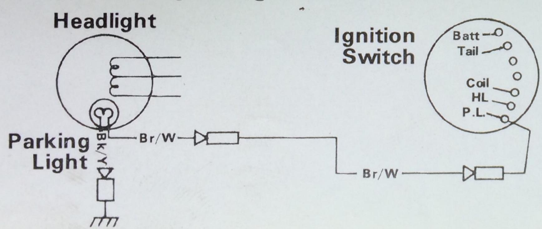
In the "Parking Lights" position, Batt, Tail, Coil and P.L. are connected inside the ignition switch.
