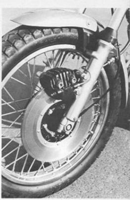
A much needed improvement this year was the addition of the single disc front brake assembly. The new lower legs are cast aluminum.
