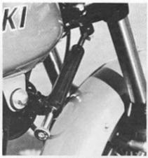
In addition to the standard friction type steering damper, Kawasaki has added a piston type damping unit underneath the lower triple clamp.
